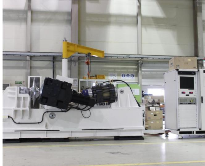
TBM Cutter Bearing Tester
